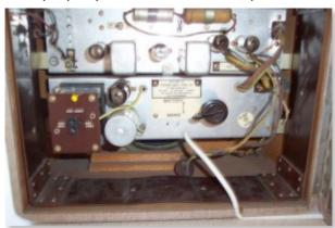
The remaining wax capacitors were tested as they were removed during the renewal process, and all proved to be leaky. The "next worst" in leakage compared to the DAF91 screen grid de-coupler was a large 0.5uF mounted on the top of the chassis, to provide AC bypass to the valve filaments. Since the set was likely to be opened frequently in order to stash the mains flex, this capacitor and a metalised paper type adjacent to it were left in situ
